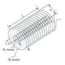
Let  $N_1$  and  $N_2$  be the total number of turns of coils S1 and S2, respectively. When a current  $I_2$  isset up through S<sub>2</sub>, it in turn sets up a magnetic flux through S<sub>1</sub>. Let us denote it by  $\Phi_1$ .
